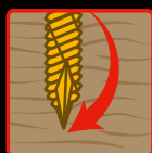
Rapid Drive Twist Cut Enhances Drive Performance
