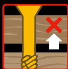
Partially Threaded Stops The Timber Jacking
